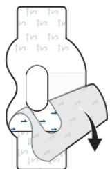
7. To apply a second tape, remove liner marked 1.
