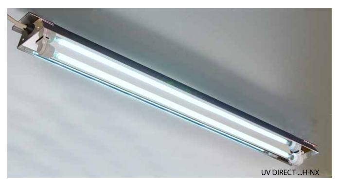
**UV-DIRECT ....H-NX** series includes a UV-C tube lodged inside a shaped case of small size, entirely made of stainless steel, and with polished aluminum screen, to increase performance also reflecting the proportion of UV-C which should be dispersed in the direction opposite to that useful . The UV-C tubes, with emission peak at 235.7 nm. (nanometers), have a strong germicidal power against all organisms (fungi, bacteria and viruses).
