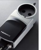
High performance progressive scan CCD camera provides quick image capture of diagnosed images and videos in real time with a simple click on joystick button.
